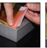
Step 1 Insert corner A Turn edge of graphic so silicon welt is perpendicular to face of graphic. Insert narrow side of welt with fabric to outside into the channel. Repeat for other side of this corne
